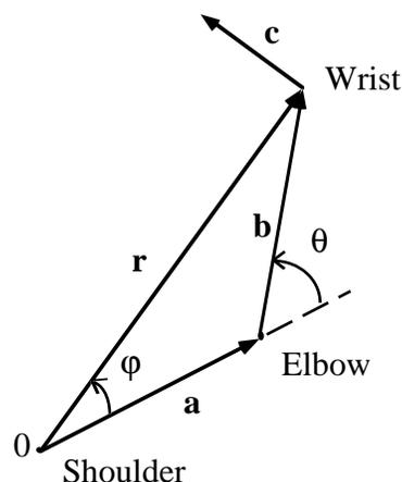
FIGURE 1. Arm configuration or posture is described by a set of relative position vectors  $\mathbf{a}, \mathbf{b}, \mathbf{c}$  relating the joints. The position of a joint is defined to be its center of rotation. The vector  $\mathbf{a}$  designates the position of the elbow relative to the shoulder;  $\mathbf{b}$  designates the position of the wrist relative to the elbow;  $\mathbf{c}$  designates the position of any point in the hand relative to the wrist.
